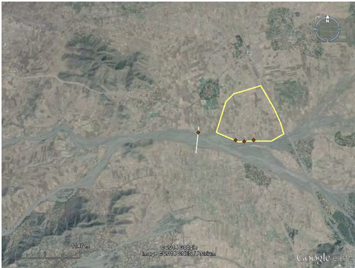
Figure 4.2 - Position of the catchment closure section (white), with the position of intakes (red) and command area (yellow) - Google Earth
